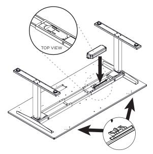
\*Control Box can be mounted in two directions, as left and right legs can be connected to either port.
