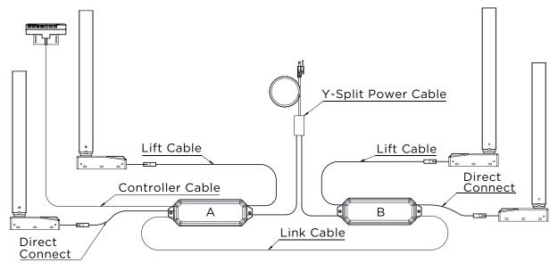
Note: Only two lift cables are needed. Two of the column cables should reach the control boxes without extra cables.
